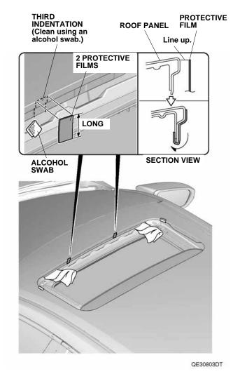
6. Remove the adhesive backing from the two protective films, and attach them to the roof panel at the third indentation.
