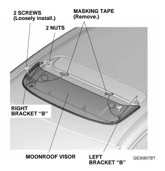
Check the information of the IMPORTANT INFORMATION label. To avoid wind noise, install the brackets against the body.
