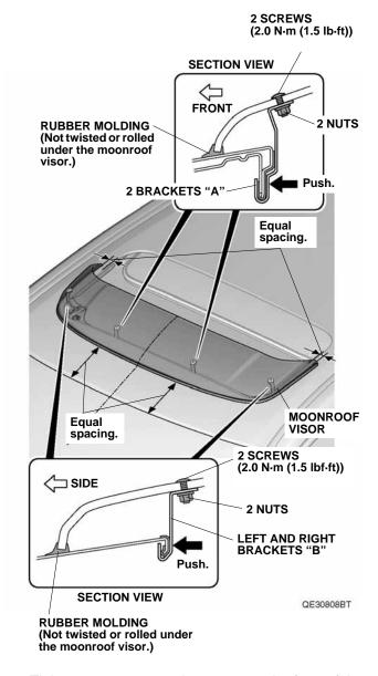
13. Tighten two screws and two nuts on the front of the vehicle first, then tighten two screws and two nuts on each side. Tighten while applying pressure so that there is no gap between the roof panel and the brackets "A" and "B". Torque the screws to 2.0 N·m (1.5 lb·ft).
