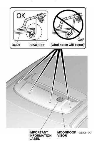
Position the moonroof visor with equal spacing in the front and on the sides. Check that the rubber molding is not twisted or rolled under the moonroof visor.
