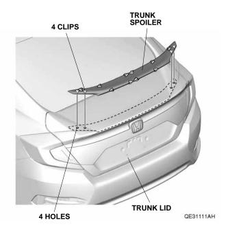
13. Adjust the position of the trunk spoiler so there is equal spacing on both sides.
