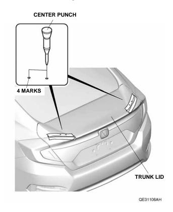
While wearing eye protection, use an 8.5 mm Rotabroach to drill four holes into the centerpunched marks. Drill perpendicular to the trunk lid.
