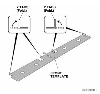
2. Line up the bottom of the template with the character line of the left front and rear doors, and line up the center hole of the template with the edge of the left front door. Then, attach the template to the left front and rear doors with masking tape as shown.
