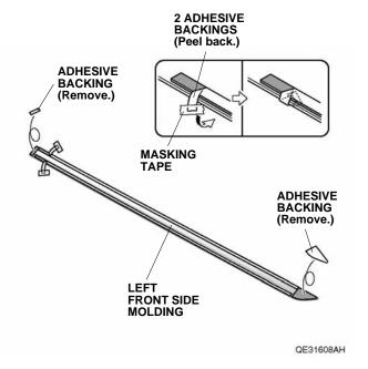
6. Line up the left front side molding with the template and install the left front side molding on the left front door.
