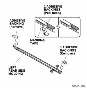
10. Line up the left rear side molding with the template and install the left rear side molding on the left rear door.
