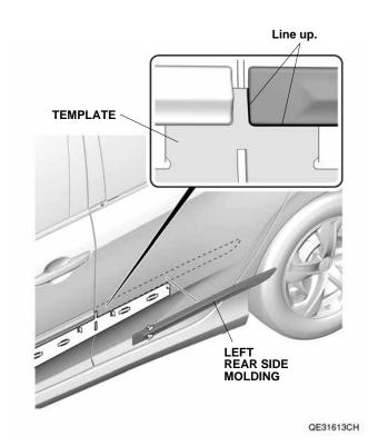
11. While applying light pressure against the left rear side molding, carefully remove the taped adhesive backings.
