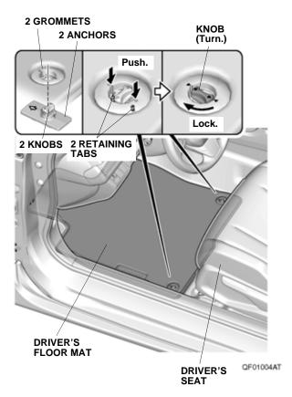
2. Place the grommets in the driver's floor mat over the anchors. Push the grommets into the anchors to secure the retaining tabs, then turn the knobs 90° to secure the driver's floor mat.
