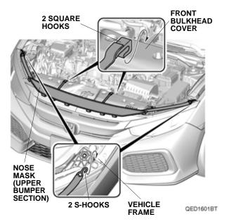
4. Attach the six hooks to the front grille opening. Insert the lower inner corner of the left tab between the front grille and front bumper, then push down and slide the tab until it's fully inserted between front grille and front bumper. Repeat for the tab on the other side.
