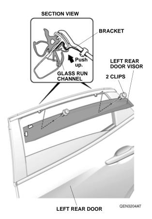
18. Secure the left rear door visor to the two brackets with the two clips. Make sure to push up on the brackets while installing the two clips.
