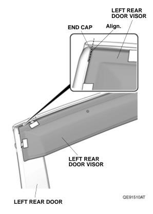
20. While applying light pressure against the left rear door visor, carefully remove the taped adhesive backings in the order shown. Make sure to push up on the brackets while removing the adhesive backings.
