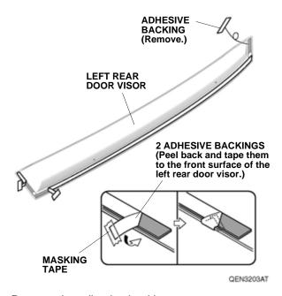
16. Remove the adhesive backing.
