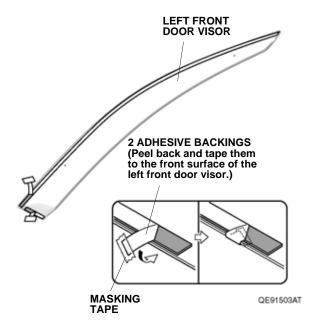
6. Line up each hole in the two brackets with the two holes in the left front door visor.
