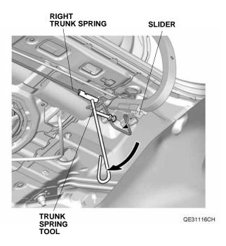
Remove the right trunk spring from the right hinge bracket.
