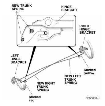
26. Install the center clip to the trunk springs.
