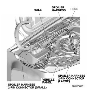
28. Unplug the vehicle 2-pin connector from the high-mount brake light connector, and plug the vehicle 2-pin connector into the spoiler harness 2-pin connector.
