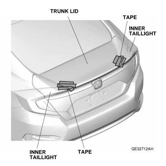
4. Place the template on the left side of the trunk lid, and line up the template with the trunk lid as shown. Tape the template to the trunk lid with masking tape.
