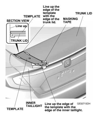
5. Using a felt-tip pen, mark the trunk lid through the template at the locations shown.
