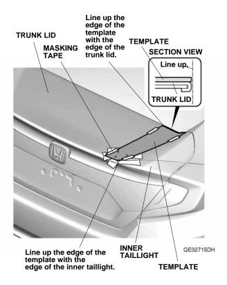
8. Using a felt-tip pen, mark the trunk lid through two outboard holes in the template.
