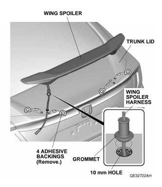
17. Remove the two adhesive backings from the wing spoiler.
