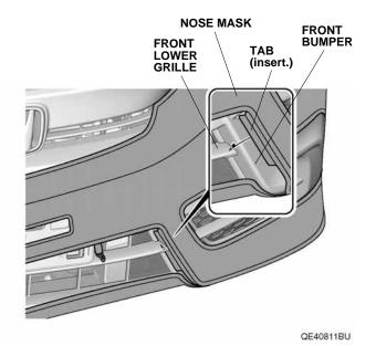
16. Attach three hooks and two S-hooks to the inside edge of the front lower grille opening as shown.
