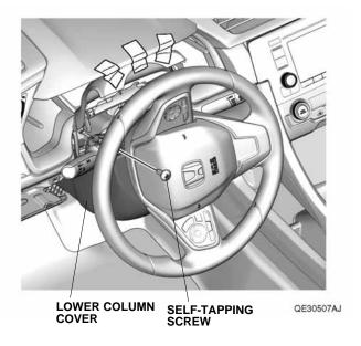
10. Turn the steering wheel 180° clockwise and remove one self-tapping screw from the lower column cover.
