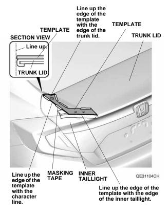
3. Using a felt-tip pen, mark the trunk lid through the template at the locations shown.
