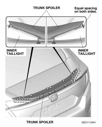
14. While applying light pressure against the trunk spoiler, carefully remove the adhesive backings as shown.
