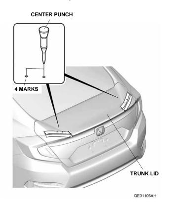
7. While wearing eye protection, use an 8.5 mm Rotabroach to drill four holes into the center-punched marks. Drill perpendicular to the trunk lid.
