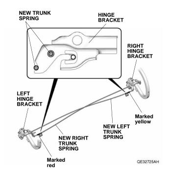
22. Install the center clip to the trunk springs.
