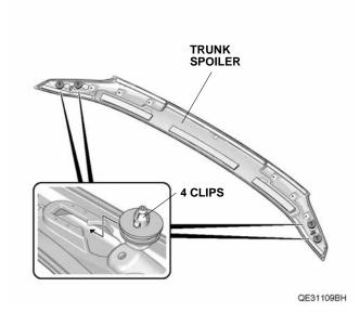
11. Using a utility knife, cut the two adhesive backings on the trunk spoiler. Peel back the adhesive backing from each adhesive strip, and tape the ends to the front surface of the trunk spoiler with masking tape.
