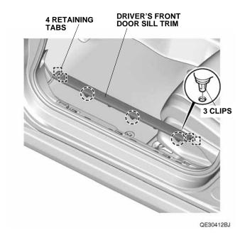
15. Pull away the door opening seal and remove the driver's kick panel.
