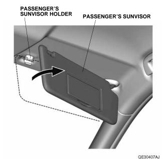
7. Remove the passenger's sunvisor holder by rotating it 90° counterclockwise.
