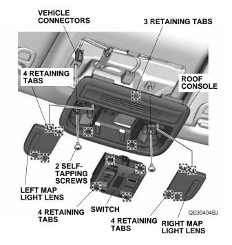
Without Moonroof and With Ambient light: Remove the roof console and unplug the vehicle connectors.
