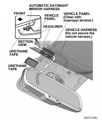
32. Secure the automatic day/night mirror harness to the vehicle panel with one urethane tape.
