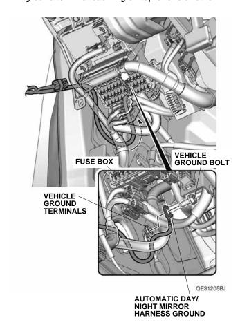
20. Secure the automatic day/night mirror harness to the vehicle harness with two wire ties.
