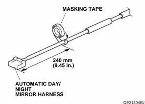
19. Remove the vehicle ground bolt and install the automatic day/night mirror harness ground terminal with vehicle ground bolt as shown. Do not put the ground terminal caulking on top of one another.
