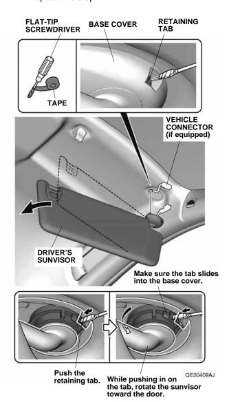
9. Remove the driver's sunvisor holder by rotating it 90° counterclockwise.
