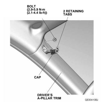
11. Pull away the door opening seal and remove the driver's A-pillar trim.
