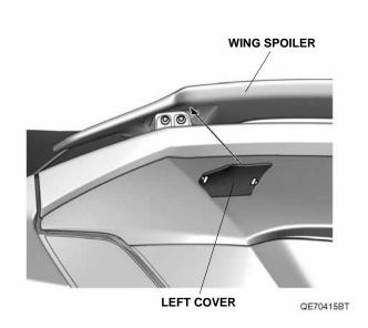
27. While applying light pressure against the left cover, carefully remove the adhesive backings as shown.
