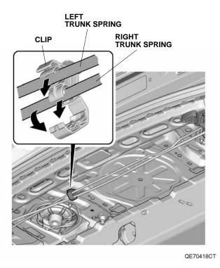
32. With an assistant holding the trunk lid open, remove the right trunk spring from the slider using the trunk spring tool. While wearing gloves to protect your hands and push down on the trunk spring tool slowly and carefully.
