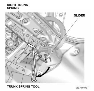
Remove the right trunk spring from the right hinge bracket.
