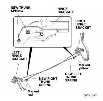
35. Install the clip to the trunk springs.
