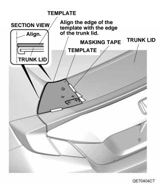
3. Using a felt-tip pen, mark the trunk lid through the template as shown.
