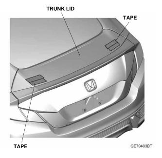
Place the template on the left side of the trunk lid and align the template with the trunk lid as shown. Tape the template to the trunk lid with strips of masking tape.
