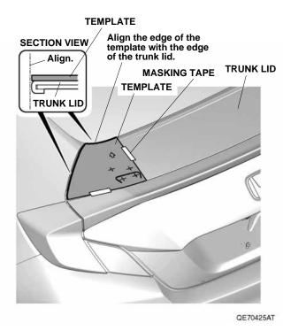
11. Using a felt-tip pen, mark the trunk lid through the template as shown.
