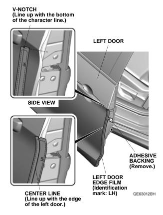
Line up the center line on the left door edge film with the edge of the left door. While applying light pressure, carefully remove the adhesive backing, and attach the left door edge film to the left door. Go to step 10.
