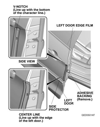
7. Line up the center line on the upper part of left door edge film with the edge of the left door. While applying light pressure, carefully remove the adhesive backing, and attach the upper part of left door edge film to the left door.
