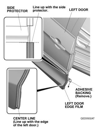
Line up the center line on the lower part of left door edge film with the edge of the left door. While applying light pressure, carefully remove the adhesive backing, and attach the lower part of left door edge film to the left door.  Insert the applicator into the soft sleeve. Starting from the top and working downward, use the soft sleeve to smooth the left door edge film. Move the soft sleeve in one direction only.
