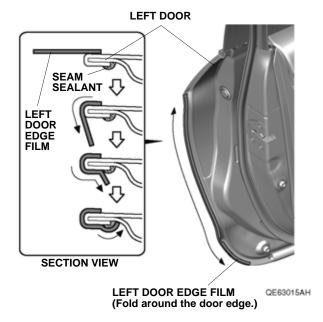
13. Using a shop towel, wipe the excess 3M protective tape application solution from the left door edge film. Allow the left door edge film to dry thoroughly.
