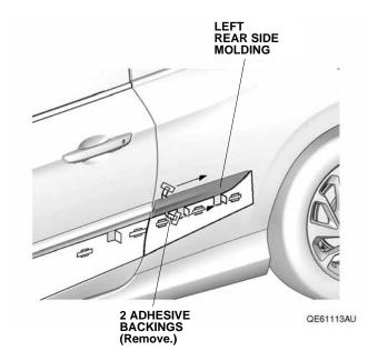
14. Using a rubber roller, apply firm pressure while rolling, especially at the ends, to set the adhesive.
