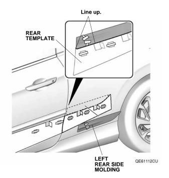
13. While applying light pressure to the left rear side molding, carefully remove the taped adhesive backings.
