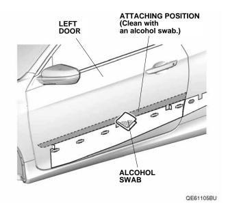
6. Using an alcohol swab, thoroughly clean the left body panel where the left rear side molding will attach.
