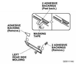
12. Line up the left rear side molding with the rear template, and attach it to the left rear panel as shown.
