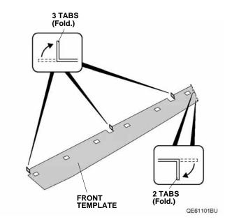
Insert the tabs on the front template between the left door and the left body panel. Line up the bottom of the front template with the character line of the left door, and attach it to the left door with masking tape.
