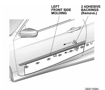
Using a rubber roller, apply firm pressure while rolling, especially at the ends, to set the adhesive.
