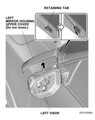
8. Install the left mirror housing upper cover to the left visor. Make sure there is no gap between the cover and the visor. Make sure to secure the retaining tabs properly.
