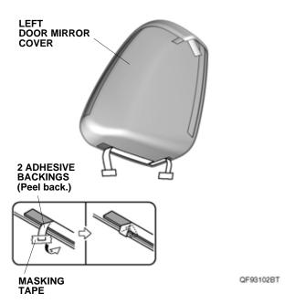
16. Using an alcohol wipe, thoroughly clean the left mirror housing upper cover where the left door mirror cover will attach.
