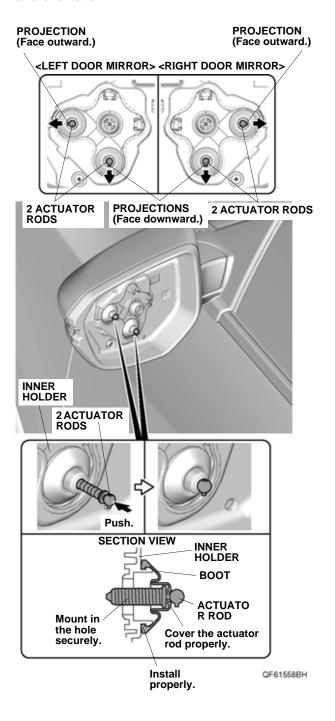
Plug the vehicle connectors into the left mirror holder (if equipped), and install the left mirror holder.
