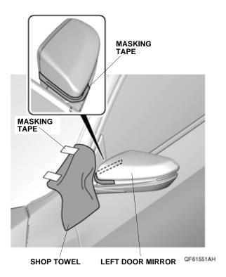
3. Release the left mirror holder. Be careful not to damage the retaining tabs.
