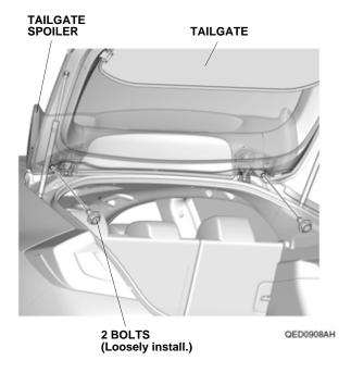
Apply pressure to the tailgate spoiler over each clip until you hear a click. Do not apply excessive pressure.
