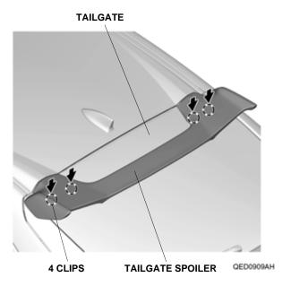
12. Hold the tailgate spoiler firmly against the tailgate over the adhesive tapes with the palm of your hand for 30 seconds.
