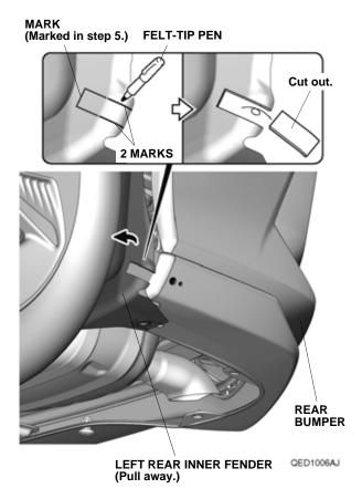
13. Using a utility knife, cut out the left rear inner fender along the marks.
