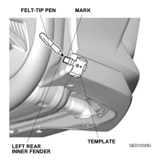
6. Using a pushpin, pierce the center of the two marks on the template.
