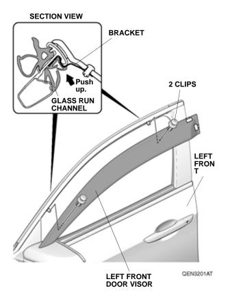
7. Secure the left front door visor to the two brackets with two clips. Make sure to push up on the brackets while installing the two clips.
