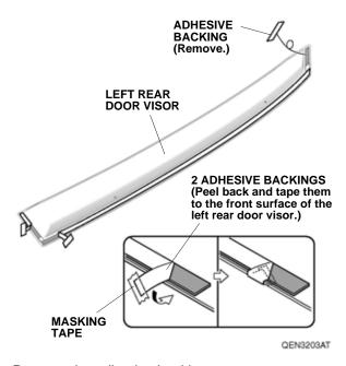
16. Remove the adhesive backing.
