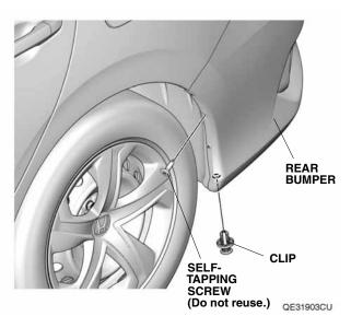
5. Locate the recessed mark. Using a pushpin, pierce the rear bumper at the recessed mark.
