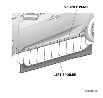
14. Attach the left spoiler to the vehicle panel with four clips.
