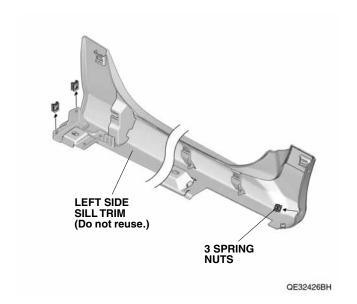
11. Install the three spring nuts on the side under spoiler as shown.
