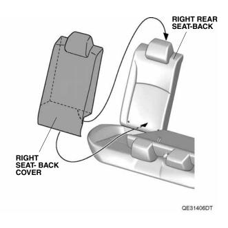
Fold down the right rear seat-back, and secure the fasteners to each other.
