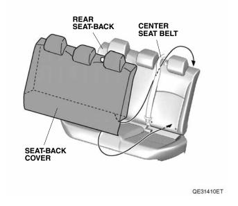
Fold down the rear seat-back, and secure the fasteners to each other.
