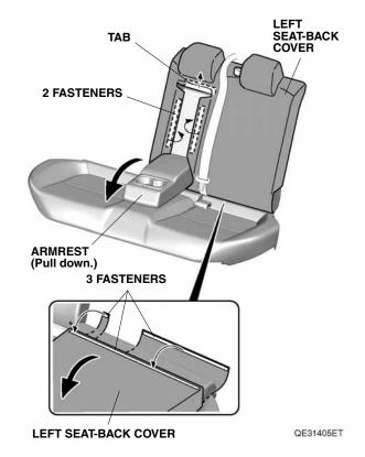
Fit the right seat-back cover onto the right rear seat-back.
