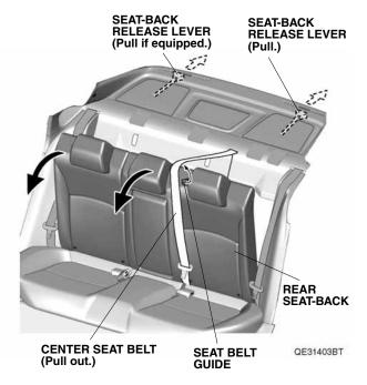
Open the trunk. Pull the seat-back release lever, and fold the rear seat-back forward.
