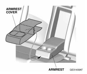
8. Raise the armrest. Pull out the armrest cover between the armrest and left rear seat-back, and secure the fasteners to each other as shown.
