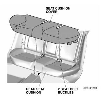
Secure the fasteners to the rear seat cushion, and insert the tabs to the rear seat cushion in the order shown
