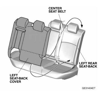
4. Pull down the armrest. Secure the fasteners to the left rear seat-back, and insert the tab in the left rear seat-back. Fold down the left rear seat-back, and secure the fasteners to each other.
