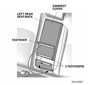
Secure the fastener to the left rear seat-back. Go to step 12.
