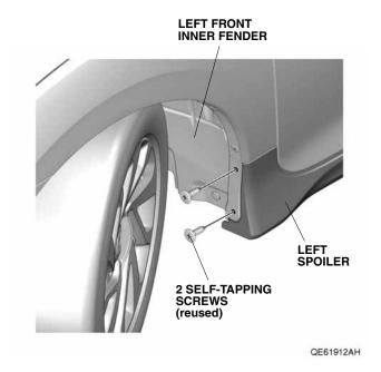
16. Secure the back of the left spoiler with two self-tapping screws.
