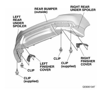
17. With the help of an assistant, install the rear bumper and left and right rear under spoilers with two hex bolts, four clips, and four self-tapping screws.
