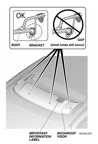
13. Position the moonroof visor with equal spacing in the front and on the sides. Check that the rubber molding is not twisted or rolled under the moonroof visor.
