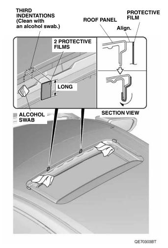
7. Remove the adhesive backing from the two protective films, and attach them to the roof panel at third indentation.
