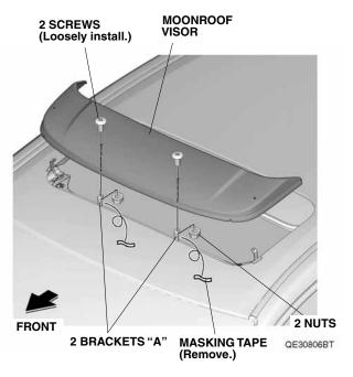
Loosely install the moonroof visor to the left and right brackets "B" with two screws and two nuts. Remove the masking tape from the left and right brackets "B".
