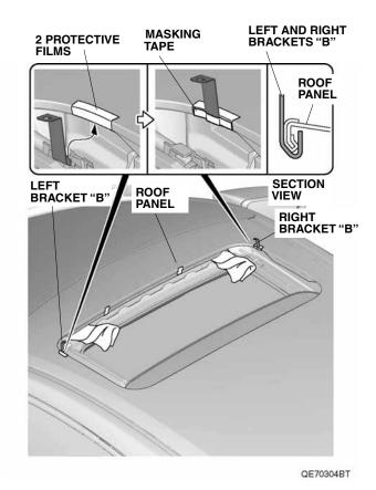
9. Place two brackets "A" into position over the two protective films and around the lip of the roof panel, and tape them into position with masking tape. Be sure to align the lower end of the brackets "A" with the third indentation.
