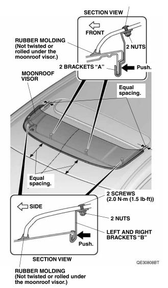
14. Tighten two screws and two nuts on the front of the vehicle first, then tighten two screws and two nuts on each side. Tighten while applying pressure so that there is no gap between the roof panel and the brackets "A" and "B". Torque the screws to 2.0 N·m (1.5 lb·ft).
