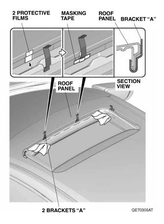
10. Set the moonroof visor on the vehicle roof in front of the moonroof opening, and adjust its position so the holes in the moonroof visor are aligned with the bracket "A" holes. Loosely install the moonroof visor to the brackets "A" with two screws and two nuts. Remove the strips of masking tape from the brackets "A".
