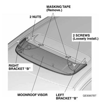
Check the information of the IMPORTANT INFORMATION label. To avoid wind noise, install the brackets against the body.
