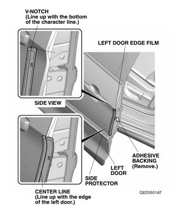
7. Line up the center line on the upper part of left door edge film with the edge of the left door. While applying light pressure, carefully remove the adhesive backing, and attach the upper part of left door edge film to the left door.
