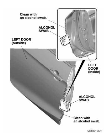
Close the left door. Using a spray bottle with 3M protective tape application solution, spray the outer area where the left door edge film will attach.
