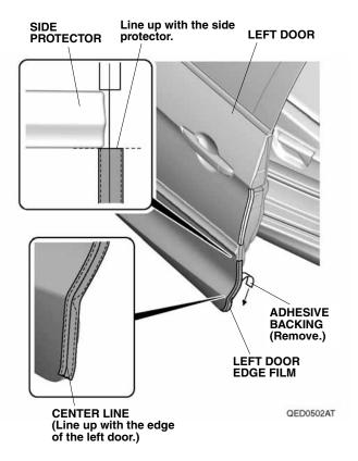
Line up the center line on the lower part of left door edge film with the edge of the left door. While applying light pressure, carefully remove the adhesive backing, and attach the lower part of left door edge film to the left door.  Insert the applicator into the soft sleeve. Starting from the top and working downward, use the soft sleeve to smooth the left door edge film. Move the soft sleeve in one direction only.
