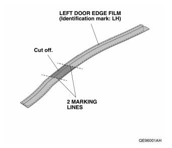
6. Open the left door. Peel back about 50 mm (1.97 in.) of adhesive backing from the upper part of left door edge film. Line up the V-notch with the bottom of the character line on the left door as shown.
