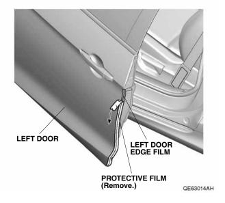
12. Starting from the center and working outward, use your fingers to fold the left door edge film around the edge of the left door as shown. Move your fingers in one direction only. Attach the left door edge film over the seam sealant. Do not trim or damage the seam sealant.
