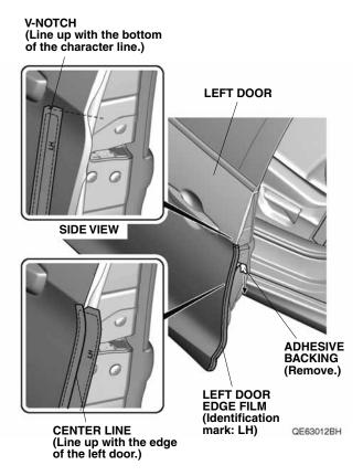
Line up the center line on the left door edge film with the edge of the left door. While applying light pressure, carefully remove the adhesive backing, and attach the left door edge film to the left door. Go to step 10.
