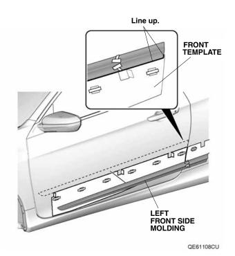
While applying light pressure to the left front side molding, carefully remove the taped adhesive backings.
