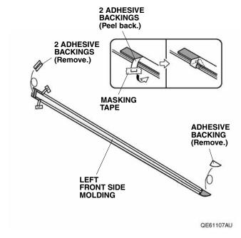
8. Line up the left front side molding with the front template and attach it to the left door as shown.
