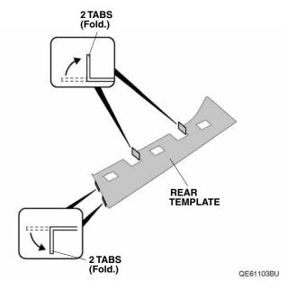
4. Insert the tabs on the rear template between the left door and the left body panel. Line up the bottom of the rear template with the character line of the left body panel, and attach it to the left body panel with masking tape.
