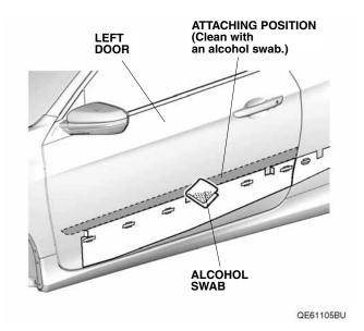
Using an alcohol swab, thoroughly clean the left body panel where the left rear side molding will attach.
