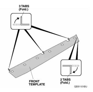
Insert the tabs on the front template between the left door and the left body panel. Line up the bottom of the front template with the character line of the left door, and attach it to the left door with masking tape.
