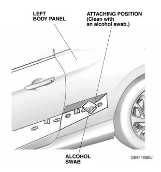
7. Peel back the adhesive backings and tape them to the front surface of the left front side molding. Remove the other adhesive backings.
