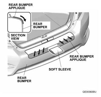
13. Using a shop towel, wipe up the 3M protective tape application solution. Allow the rear bumper applique to dry thoroughly. Remove the masking tape.
