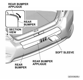
12. Repeat step 9 at the left and right sides of the lower section on the rear bumper applique.
