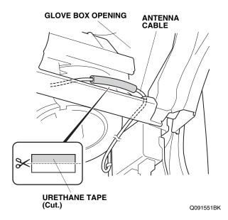
Secure the antenna cable to the vehicle frame with one wire tie.
