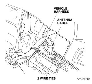
44. Secure the antenna cable to the vehicle panel with one wire tie with clip in the area shown.
