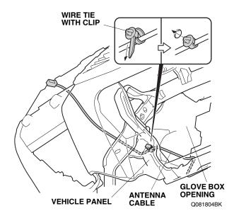
45. Secure the antenna cable to the vehicle frame with two wire ties.
