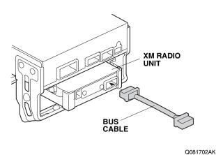
30. Plug the 2-port bus cable into the audio unit connector and the bus cable connector.
