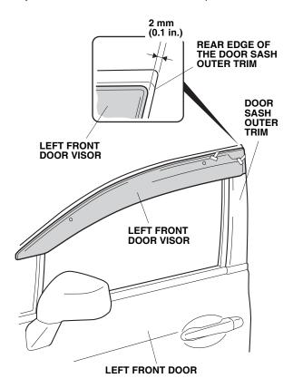
While applying light pressure against the left front door visor, carefully remove the adhesive backings. Use your finger to push up each bracket so there is no gap between the brackets and the door sash.
