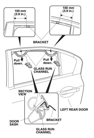
Install two brackets between the door sash and the glass run channel at the measurements shown. Seat the glass run channel properly around the brackets. 14. Using isopropyl alcohol on a shop towel, thoroughly clean the area where the left rear door visor will attach.
