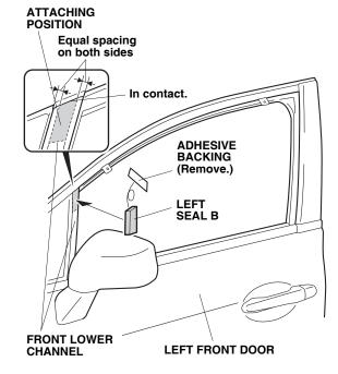
Remove the adhesive backing from the seal A, and attach it to the door sash in the area shown.
