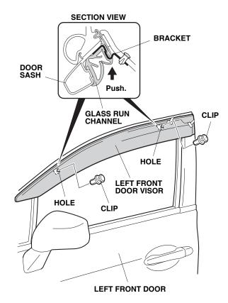
8. Adjust the left front door visor to the position shown.
