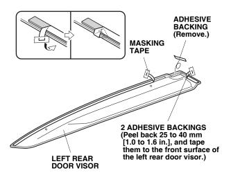
17. Align the clip holes in the left rear door visor with the bracket holes, and install the two clips. There should be no clearance between the brackets and the door sash.
