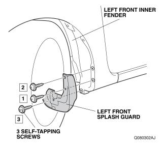
4. Turn the steering wheel fully clockwise, and repeat steps 2 and 3 to install the right front splash guard on the right side of the vehicle.
