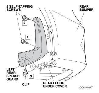
Turn the template over, and repeat steps 5 through 13 to install the right rear splash guard on the right side of the vehicle.
