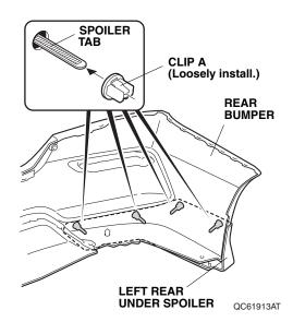
12. Remove three adhesive backings in the order shown. Press the left rear under spoiler firmly against the rear bumper with the palm of your hand for 30 seconds to adhere the left rear under spoiler.
