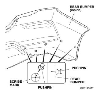
3. While wearing eye protection, drill the lower pierced mark with a 3 mm drill bit, with a 6 mm drill bit, with an 8 mm drill bit, then finish with a 10 mm drill bit. Repeat on the other side of the rear bumper.
