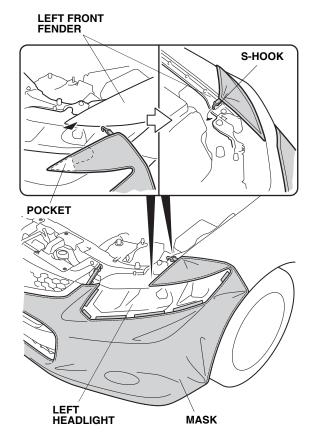
8. Attach the S-hook to the mask on the left front fender.
