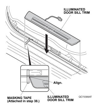
40. Route the illuminated door sill trim harness over the vehicle panel of the door opening seal.
