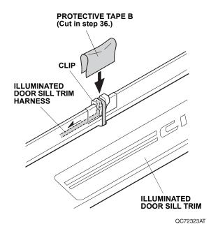
65. Plug the illuminated door sill trim harness 2-pin connector into the door sill trim harness 2-pin connector.
