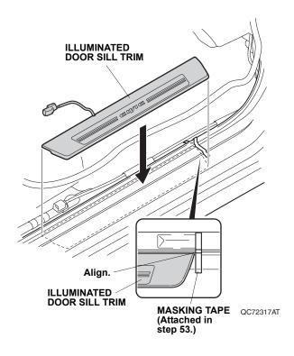
55. Route the illuminated door sill trim harness over the vehicle panel of the door opening seal.
