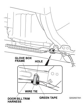
31. Secure the door sill trim harness to the glove box frame with one wire tie.
