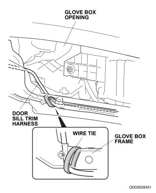
32. Inside the center lower panel opening, secure the door sill trim harness to the vehicle harness with two wire ties.
