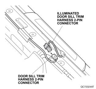
66. Bundle up the excess illuminated door sill trim harness, and secure it to the vehicle harness with one wire tie with holder.
