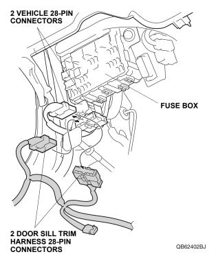
20. Attach the door sill trim harness 28-pin connector to the vehicle 28-pin connector.
