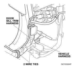
24. Continue to route the door sill trim harness along the vehicle harness, then loop the connector back to the measurement shown. Secure the door sill trim harness to the vehicle harness with three wire ties.
