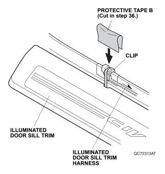
Plug the illuminated door sill trim harness 2-pin connector into the door sill trim harness 2-pin connector.
