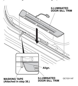
47. Attach the illuminated door sill trim to the vehicle panel by removing five adhesive backings in the order shown and pressing on the trim firmly with your hands.
