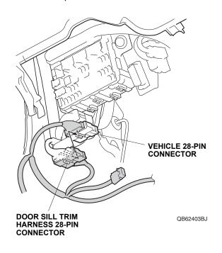
21. Attach the door sill trim harness fuse case to the bottom of the fuse box.
