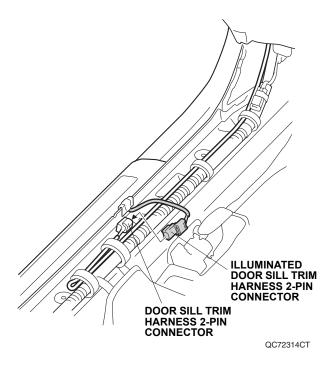
51. Bundle up the excess illuminated door sill trim harness, and secure it to the vehicle harness with one wire tie with holder.
