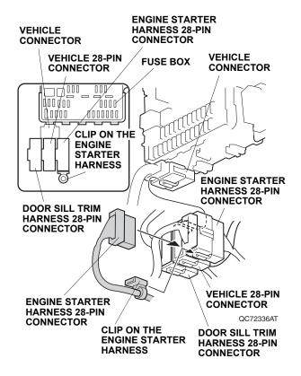
16. Remove the connectors and clip on the engine starter harness as shown. Unplug the engine starter harness 28-pin connector from the engine starter harness 28-pin connector, and the vehicle 28-pin connector from the vehicle 28-pin connector.
