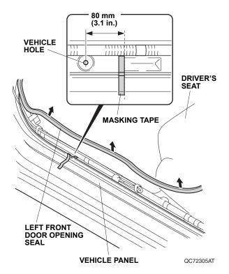
38. Attach a strip of masking tape to the vehicle panel at the location shown.
