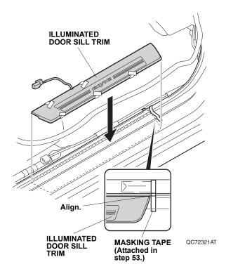
62. Attach the illuminated door sill trim to the vehicle panel by removing five adhesive backings in the order shown and pressing on the trim firmly with your hands.
