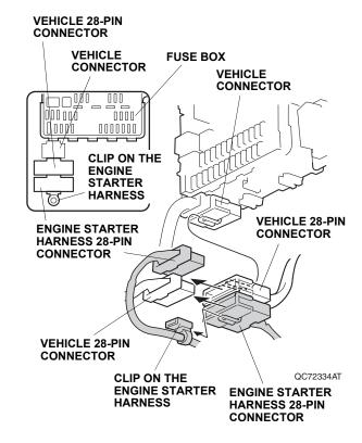
14. Plug the door sill trim harness 28-pin connector into the engine starter harness 28-pin connector. Plug the vehicle 28-pin connector into the remaining door sill trim harness 28-pin connector, and attach them to the vehicle 28-pin connector.
