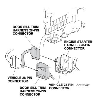
Plug the engine starter harness 28-pin connector into the engine starter harness 28-pin connector.
