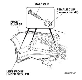
15. Remove two adhesive backings in the order shown. Press the left front under spoiler firmly against the front bumper with the palms of your hands to adhere the left front under spoiler.
