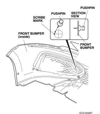
7. Using a pushpin, pierce three scribe marks on the front bumper as shown.
