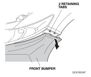
• On each side, release four retaining tabs.
