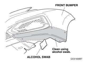
Peel back about 40 to 50 mm (1.6 to 2.0 in.) of adhesive backing from each adhesive strip, and tape the ends to the front surface of the left front under spoiler.
