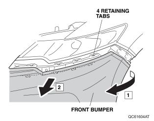
With the help of an assistant, remove the front bumper (four clips and unplug the vehicle connectors). Place the front bumper on a blanket to prevent damage.
