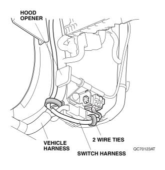
55. Secure the switch harness to the vehicle harness with two wire ties.
