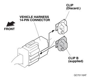
43. Unplug the vehicle harness 14-pin connector.
