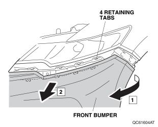
With the help of an assistant, remove the front bumper (four clips). Place the front bumper on a blanket to prevent damage.
