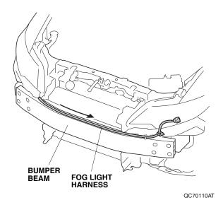
Secure the fog light harness clip to the hole in the extension as shown.
