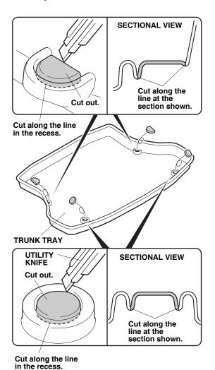
2. Open the trunk lid. Place the trunk tray on the trunk floor.
