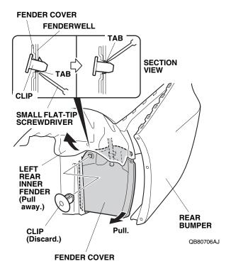
12. Working inside the fenderwell, use a small flat-tip screwdriver to release the tabs on the clip, then remove the clip with a trim tool.
