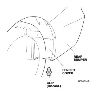
10. Pull the rear bumper away from the body, and release the seven retaining tabs.
