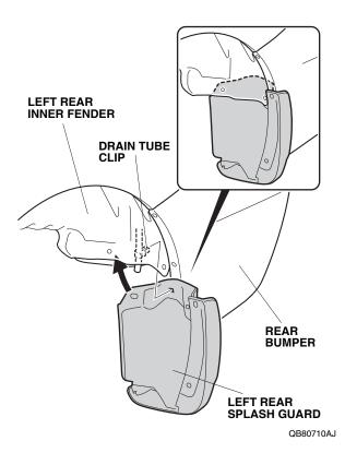
30. Secure the left rear splash guard with two 5 x 25 mm self-tapping screws and one 5 x 30 mm self-tapping screw in the order shown below.
