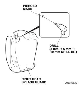
34. Remove any burrs from the edges of the hole with a file.
