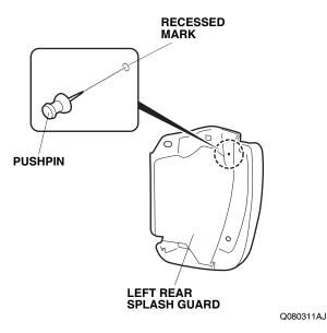
6. While wearing eye protection, drill the left rear splash guard at the pierced mark using a 3 mm drill bit first, then with a 6 mm drill bit. Finish drilling using a 10 mm drill bit.
