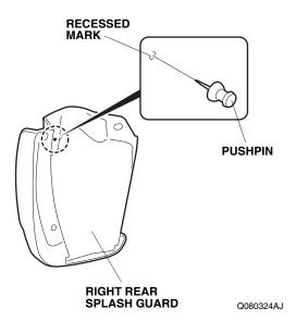
33. While wearing eye protection, drill the right rear splash guard at the pierced mark using a 3 mm drill bit first, then with a 6 mm drill bit. Finish drilling using a 10 mm drill bit.
