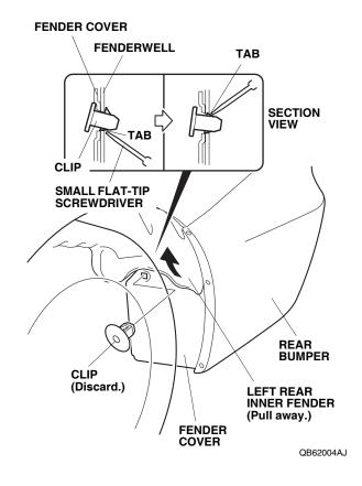
23. Remove the fender cover (one drain tube clip).
