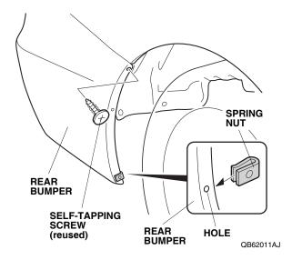
41. Install one spring nut over the hole in the rear bumper. Make sure to install the spring nut in the correct position and orientation.
