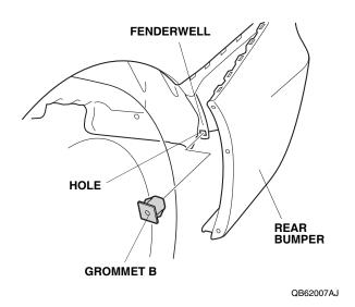
27. Reinstall the rear bumper onto the retaining tabs, and reinstall one self-tapping screw.
