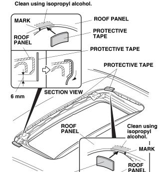
5. Remove the adhesive backings from two pieces of protective tape, and attach them to the roof panel at the two marks you made. Allow 6 mm of each protective tape to hang below the bottom lip of the roof panel. Remove the marks.
