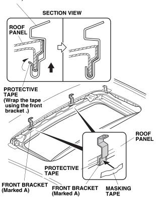
10. Using 3M protective tape application solution, spray the roof in the area shown where the moonroof visor will attach.
