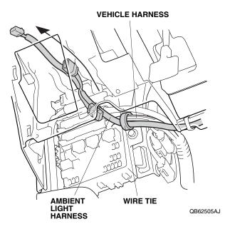
11. Route the ambient light harness up to the switch lid opening, and secure it to the vehicle harness with two wire ties.
