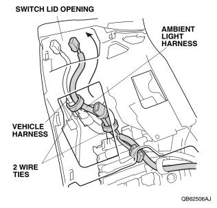
12. Unplug the vehicle 6-pin (5-pin on Si model) connector from the switch, and plug it into the ambient light harness 6-pin (5-pin on Si model) connector.
