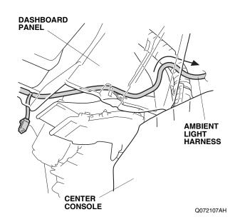
15. Secure the ambient light harness to the vehicle frame with one wire tie.
