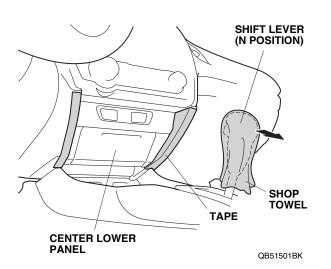
5. Remove the center lower panel (two self-tapping screws, four clips, and unplug the vehicle connectors, if equipped).
