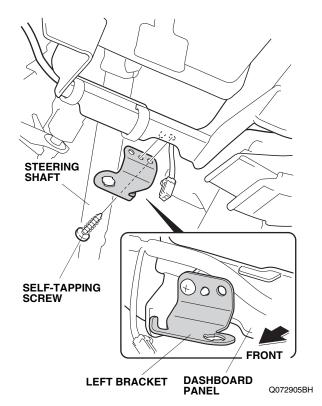
23. Install the ambient light to the left bracket by rotating it into position.
