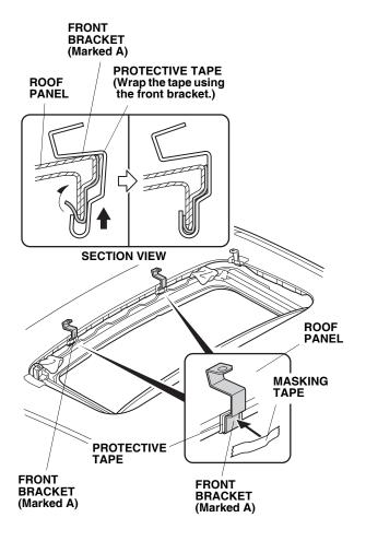
11. Set the moonroof visor on the vehicle roof in front of the moonroof opening, and adjust its position so the holes in the moonroof visor are aligned with the bracket holes. Loosely install the moonroof visor onto the front bracket (marked A) with two screws and two nuts. Remove the masking tape.
