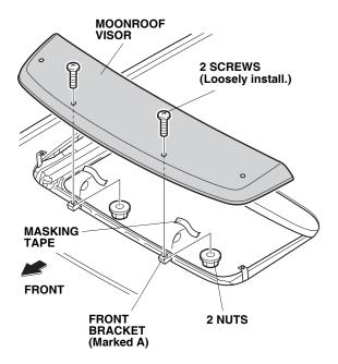
12. Loosely install the moonroof visor to the side brackets (marked B) with two screws and two nuts. Remove the masking tape.
