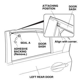
16. Peel back about 25 to 40 mm (1.0 to 1.6 in.) of adhesive backing from each adhesive tape, and tape the ends to the front surface of the left rear door visor. Remove the other adhesive backing.
