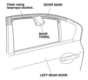
15. Remove the adhesive backing from seal A, and attach it to the door sash.
