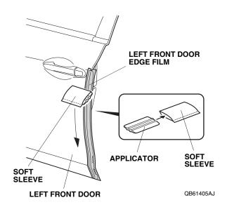
6. Slowly remove the protective film from the left front door edge film.
