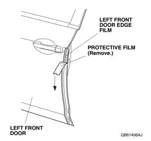
7. Starting from the center and working outward, use your fingers to fold the left front door edge film around the edge of the left front door as shown. Move your fingers in one direction only. Attach the left front door edge film over the seam sealant. Do not trim or damage the seam sealant.
