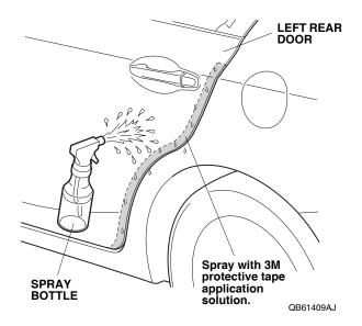
Open the left rear door. Peel back about 50 mm (2.0 in.) of adhesive backing from the left rear door edge film. Align the V-notch 50 mm (2.0 in.) above the character line on the upper part of the left rear door as shown.
