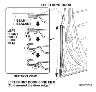
Using a shop towel, wipe the excess 3M protective tape application solution from the left front door edge film. Allow the left front door edge film to dry thoroughly.
