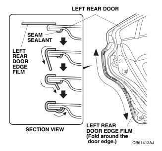
15. Using a shop towel, wipe the excess 3M protective tape application solution from the left rear door edge film. Allow the left rear door edge film to dry thoroughly.
