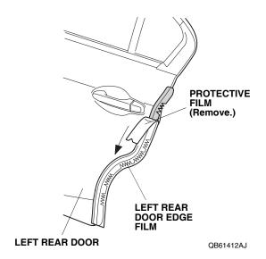
14. Starting from the center and working outward, use your fingers to fold the left rear door edge film around the edge of the left rear door as shown. Move your fingers in one direction only. Attach the left rear door edge film over the seam sealant. Do not trim or damage the seam sealant.
