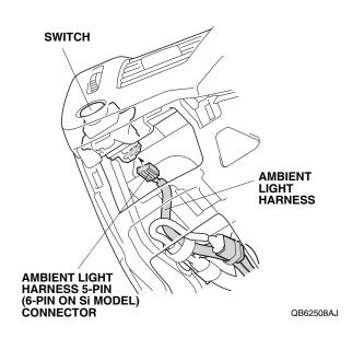
14. Route the ambient light harness 2-pin connector toward the passenger's side of the vehicle.
