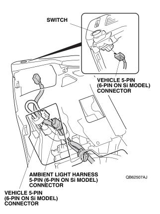
13. Plug the ambient light harness 5-pin (6-pin on Si model) connector into the switch.
