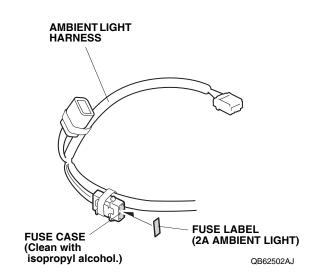
7. Attach the fuse label (2A AMBIENT LIGHT) to the ambient light harness fuse case.
