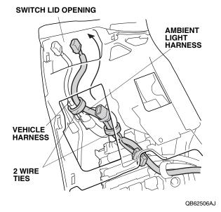
12. Unplug the vehicle 5-pin (6-pin on Si model) connector from the switch, and plug it into the ambient light harness 5-pin (6-pin on Si model) connector.
