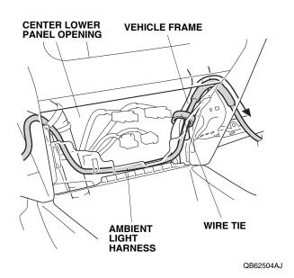
18. Inside the glove box opening, secure the ambient light harness with one wire tie at the location shown.
