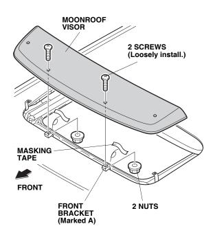
Loosely install the moonroof visor to the side brackets (marked B) with two screws and two nuts. Remove the masking tape.
