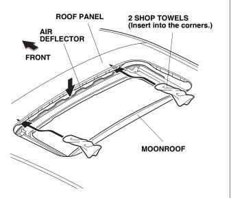
3. Locate the edge of the indentation on the right side and left side of the moonroof opening. Measure 45 mm to the front of the vehicle, and make two marks on the roof panel.
