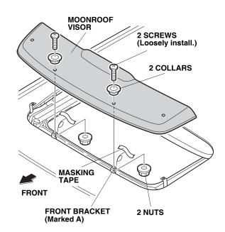
Loosely install the moonroof visor to the side brackets with two screws, two collars, and two nuts. Remove the masking tape.
