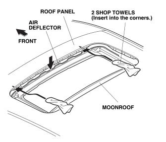
Locate the edge of the indentation on the right side and left side of the moonroof opening. Measure 45 mm to the front of the vehicle, and make two marks on the roof panel.
