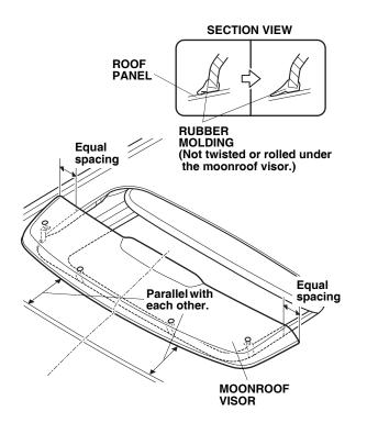
14. Tighten two screws and two nuts on the sides of the visor first, then tighten two screws and two nuts on the front. Tighten while applying pressure so that there is no gap between the roof panel and the brackets. Torgue the screws to 2.0 N·m (1.5 lbf·ft).
