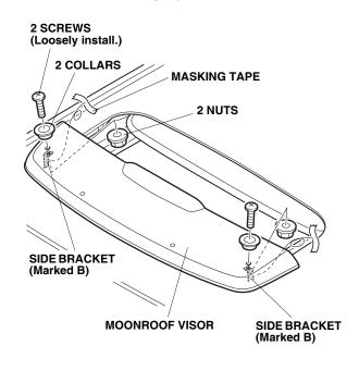
13. Position the moonroof visor with equal spacing on all sides. Check that the rubber molding is not twisted or rolled under the moonroof visor.
