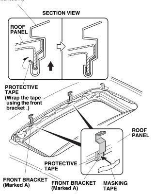
11. Set the moonroof visor on the vehicle roof in front of the moonroof opening, and adjust its position so the holes in the moonroof visor are aligned with the bracket holes. Loosely install the moonroof visor to the front brackets with two screws, two collars, and two nuts. Remove the masking tape.
