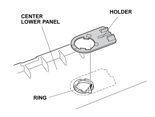
27. Secure the ambient light to the holder by rotating it into position. Go to step 34.
