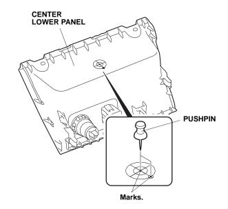
23. While wearing eye protection, drill the two pierced marks with a 3 mm drill bit. Enlarge one 3 mm hole with a 20 mm hole saw.
