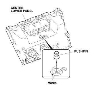
29. While wearing eye protection, drill the two pierced marks with a 3 mm drill bit. Enlarge one 3 mm hole with a 20 mm hole saw.
