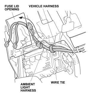
19. Using one wire tie, secure the ambient light harness to the vehicle harness.
