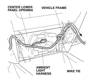
15. Using one wire tie, secure the ambient light harness to the vehicle frame.
