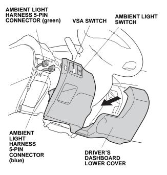
49. Reinstall the driver's dashboard lower cover. Go to step 55.
