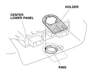
33. Secure the ambient light to the holder by rotating it into position.
