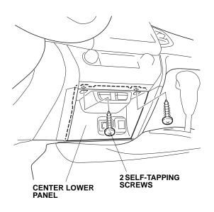
5. Remove the center lower panel (three clips, one retaining tab, and unplug the vehicle connectors).
