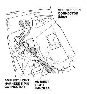
48. Plug the ambient light harness 5-pin connector (blue) into the ambient light switch, and plug the harness 5-pin connector (green) into the VSA switch.
