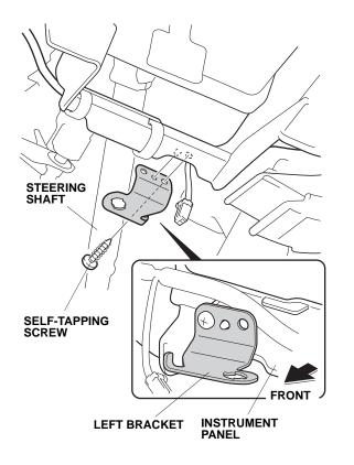
39. Install the ambient light to the left bracket by rotating it into position.
