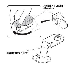
36. Plug the ambient light harness 2-pin connector into the ambient light.
