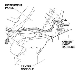
12. Using one wire tie, secure the ambient light harness to the vehicle frame.
