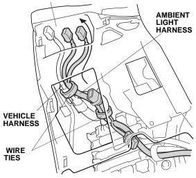
21. Using two wire ties, secure the ambient light harness to the vehicle harness.
