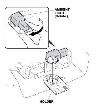
34. Plug the ambient light harness 2-pin connector into the ambient light, and reinstall the center lower panel.
