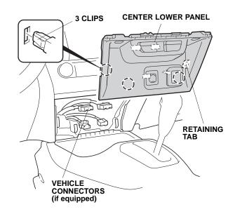
6. Remove the driver's dashboard lower cover (nine clips and unplug the vehicle connector, if equipped).
