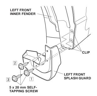
4. Turn the steering wheel all the way clockwise, and repeat steps 2 and 3 to install the right front splash guard.
