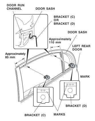
Position the left rear door visor on the door sash.
