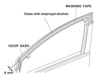
27. Peel back 1½ to 2 inches of adhesive backing from each adhesive tape, and tape the ends to the front surface of the door visor with masking tape..
