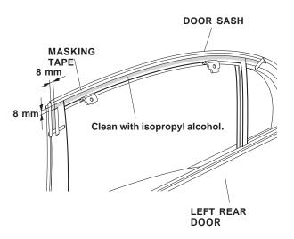
11. Peel back 1½ to 2 inches of adhesive backing from each adhesive tape, and tape the ends to the front surface of the door visor with masking tape.
