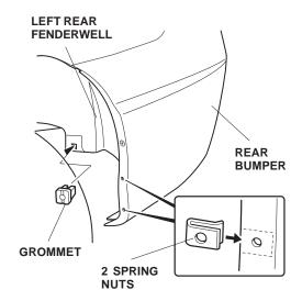
7. Position the left rear splash guard on the left rear fenderwell and rear bumper, then install the three 5 x 20 mm self-tapping screws. Tighten the three self-tapping screws in the order shown. Cut off any excessive undercoat material with a utility knife.
