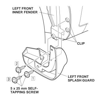
4. Turn the steering wheel all the way clockwise, and repeat steps 2 and 3 to install the right front splash guard.
